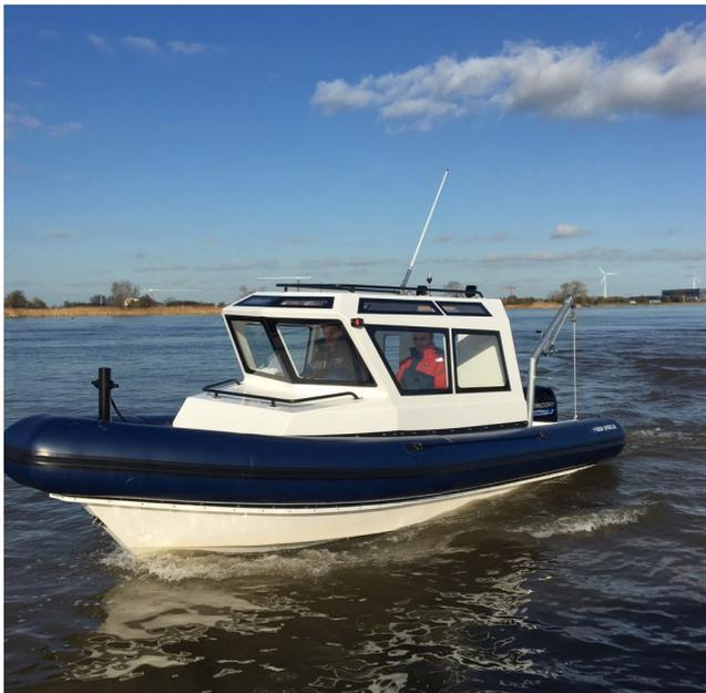
Example: BS 6.5 cabin complete with Mercury Seapro 150 HP, three jockey seats, navigation lights, work-lights, bollard, ready to sail. Also available with OXE 125 HP outboard Diesel or
